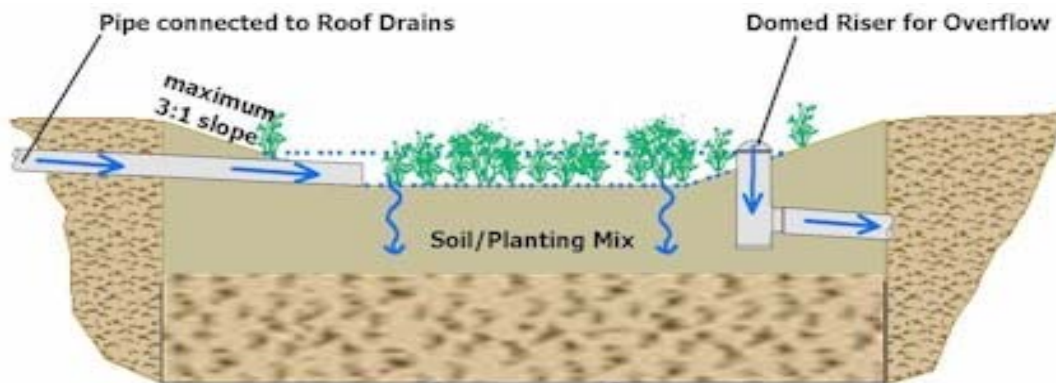
Figure 4: Cross-Section of Typical Rain Garden/Bioretention Area
